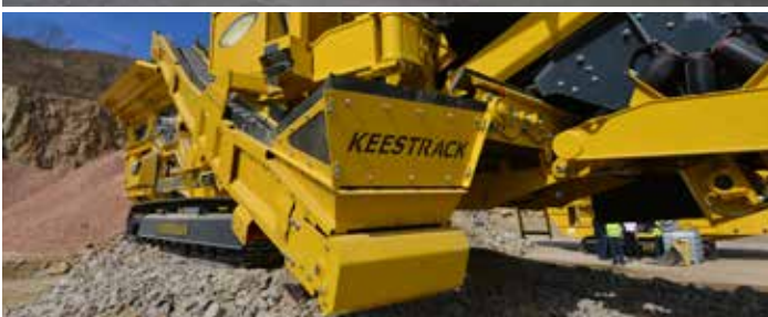
Swiveling return/stockpile conveyor
