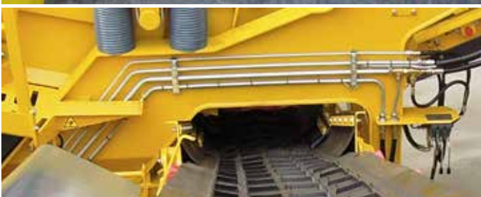
Steel hydraulic lines
