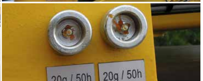
Protected greasing nipples
